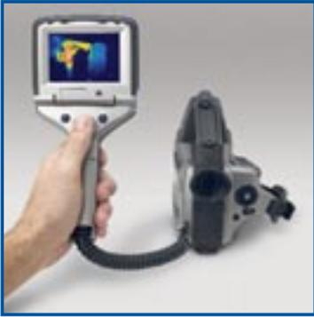
*Detachable LCD and remote control allow you to view images and control functions while the camera is positioned in hard-to-reach areas—both indoors and outside.*
