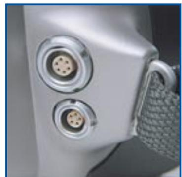
*USB, RS 232 connections for fast downloads of 14-bit JPEG images with measurements.*
