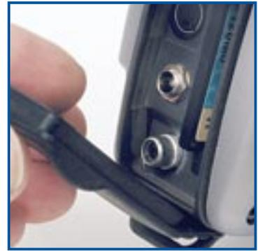
*Fast access to composite and S-video connections.*
